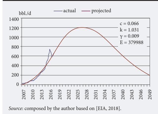
Figure 10. Main models based on the differential oil production balance equation
